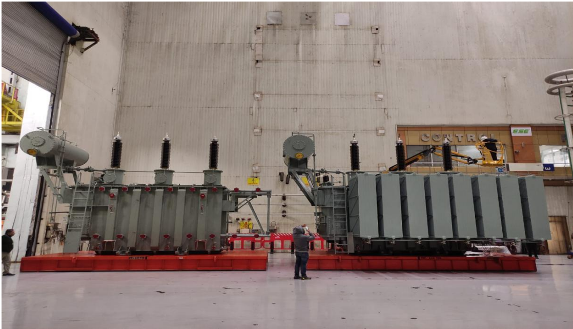
FAT test of unit 1 and unit 2 Power Transformers held at Shirdi Sai Electricals Limited at Naini, Prayagraj
